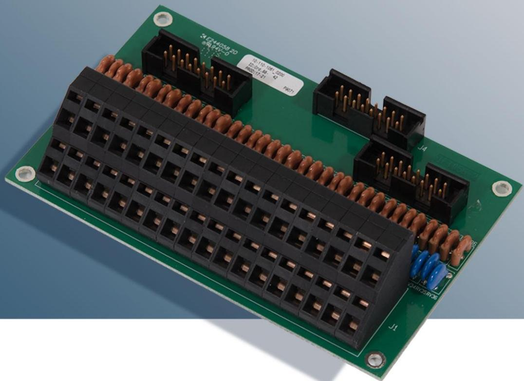
18 line Cable Termination Unit: 16 extensions + 2 trunk lines.
