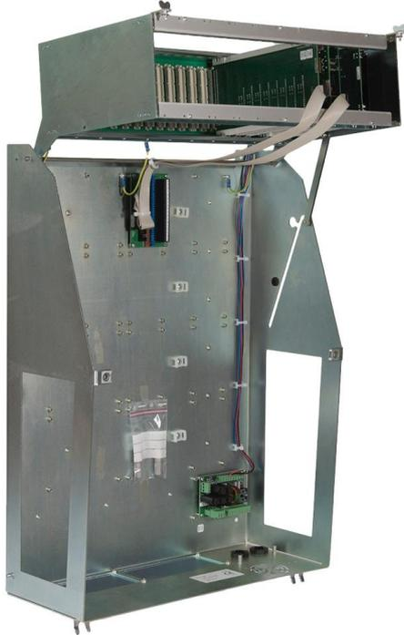
The system is powered from 24V DC, and there are two inputs - main and battery.
