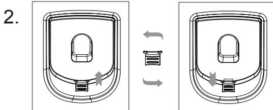
rotate the receiver suspension tab 180° according to the picture; this tab will hold the receiver when used in a suspended position
