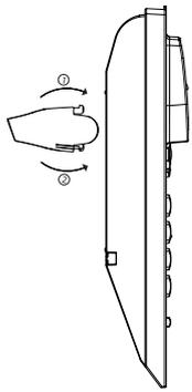
you can use the phone as a desk model by clicking the bracket onto the bottom of the phone according to the illustration below
