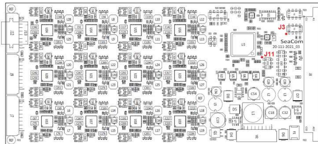
To the left, the 3 lines connectors are found. These have the 2 wire analogue telephone lines.
