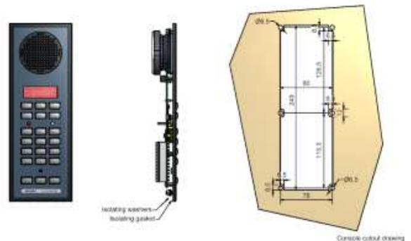
It is important to make a precise cutout, in order to be able to make the required electrical isolation between the station and the steel of the console.
