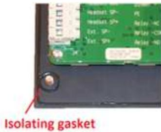
And it is supplied with 6 isolation washers (“hats”), which are used when mounting the nuts from behind.
