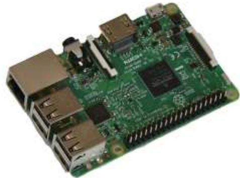
The LSP is a power full 64bit quad core 1.2 GHz computer, that takes care of being the "brain" of the SeaCom 3000.
