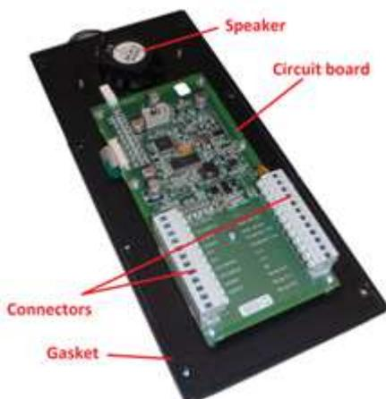
The picture show the connectors without the cable part to which the ship cables are connected.
