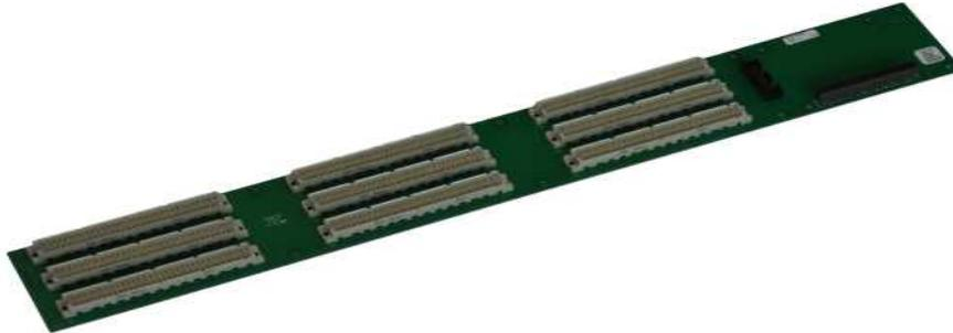
The purpose of the backplane is to interconnect all circuit boards, and to distribute power. The backplane also carries the LSP board.
