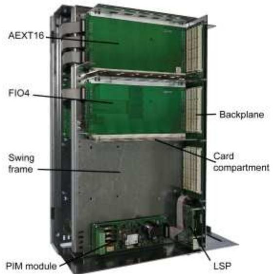
The system is two layered. The figure above shows the swing frame layer, holding all circuit boards.
