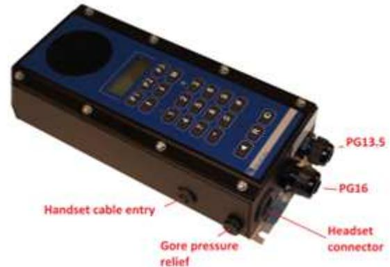
The box is watertight due to the use of PG cable entries with O-rings. Openings optionally used, are on delivery closed by grommets, which are removed when the handset or headset is to be attached to the station. There are two optional cable inlets for the handset and for the headset water tight connector set.
