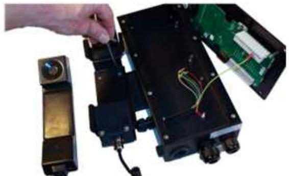
Tighten the PG9 cable gland so it forms a water tight cable pass through, and put on the ferrite delivered with the handset.
