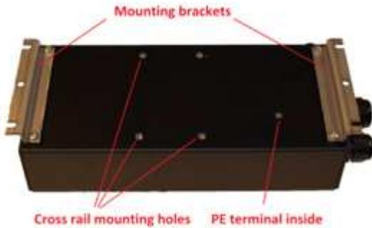
These are used for hanging the station on a bulkhead. In order to make it legal to terminate the cable shield to the PE terminal of the encapsulation, the two stainless mounting brackets are isolated from the aluminum box by isolating washers as seen on the below picture.
