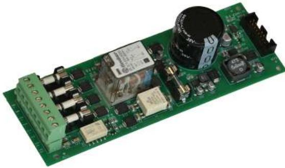
The PIM is used to connect 24V DC to power the system. It holds the main fuses, and it holds the switch over circuit responsible for switching to the backup power supply when main power fails.
