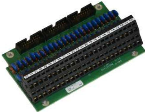
The CTU24 is used to be the interface between the ribbon cables and the ship cables. And it takes care of being the EMC barrier of the system shorting transients and lightning to the basis frame of the cabinet.
