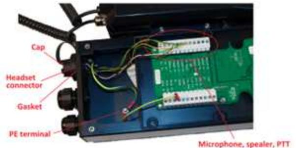
The headset with the cable part water tight connector is now ready to be attached to the station when installed.
