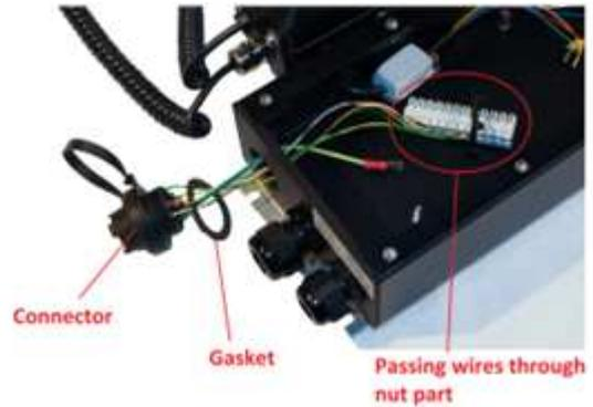
Connector, Gasket, Passing wires through nut part
