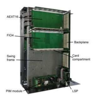
The system is two layered. The figure above shows the swing frame layer, holding all circuit boards.
