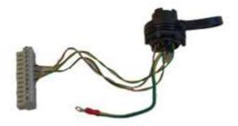
Remove the grommet covering the headset connector hole.
