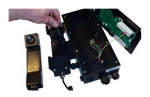
Tighten the PG9 cable gland so it forms a water tight cable pass through, and put on the ferrite delivered with the handset.
