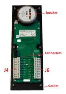
The picture shows the station without the shielding mounted, so that the PCB can be seen.
