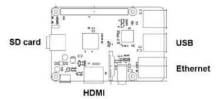
To the left, the SD card connector is found. this card is the "hard disk" of the system, holding the Linux operating system, and all the required system software and files.
