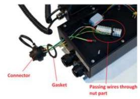
Tighten the nut, connect the PE terminal and connect the PCB connector part to the PCB.
