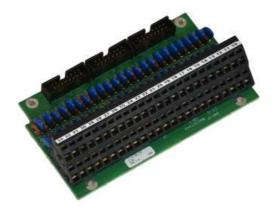
The CTU24 is used to be the interface between the ribbon cables and the ship cables. And it takes care of being the EMC barrier of the system shorting transients and lightening to the basis frame of the cabinet.
