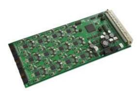
The AEXT16 is the telephone line card of the system. The AEXT16 that comes with the SeaCom 3000 has 24 lines, but the AEXT16 line card comes in 8 or 16 lines versions as well, in order to more closely adapt the need of the single customer.
