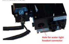
Pass the white connector through the hole, and make sure that the gasket is in place.
