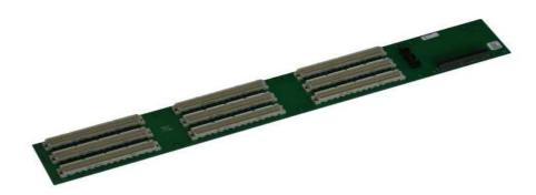
The purpose of the backplane is to interconnect all circuit boards, and to distribute power. The backplane also carries the LSP board.
