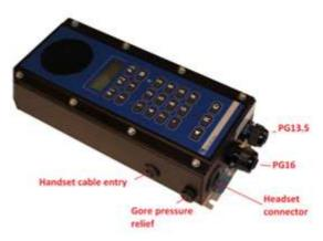
The box is watertight due to the use of PG cable entries with O-rings. Openings optionally used, are on delivery closed by grommets, which are removed when the handset or headset is to be attached to the station. There are two optional cable inlets for the handset and for the headset water tight connector set.
