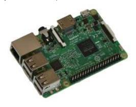
The LSP is a power full 64bit quad core 1.2 GHz computer, that takes care of being the "brain" of the SeaCom 3000.
