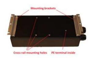
These are used for hanging the station on a bulkhead. In order to make it legal to terminate the cable shield to the PE terminal of the encapsulation, the two stainless mounting brackets are isolated from the aluminum box by isolating washers as seen on the below picture.
