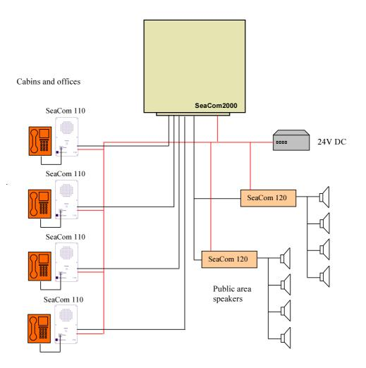
Figure 2. Typical SeaCom2000 public address installation. The red lines are 24V DC power lines. The black lines are extension lines. Note that more than one SeaCom 120 can be connected to one extension line.
