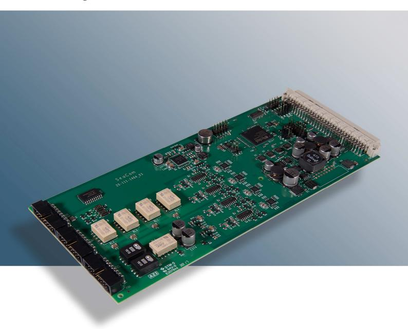
2 or 4 line trunk card used for all SeaCom exchange systems. Includes 2 audio I/O.
