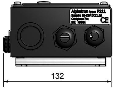
Mounting will ensure isolation between ship hull and the aluminium box of the communication station. Cable shields are to be terminated at the PE terminal inside station.
